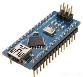
Figura 1. Arduino nano ATmega328P [Filipeflop 2018]
